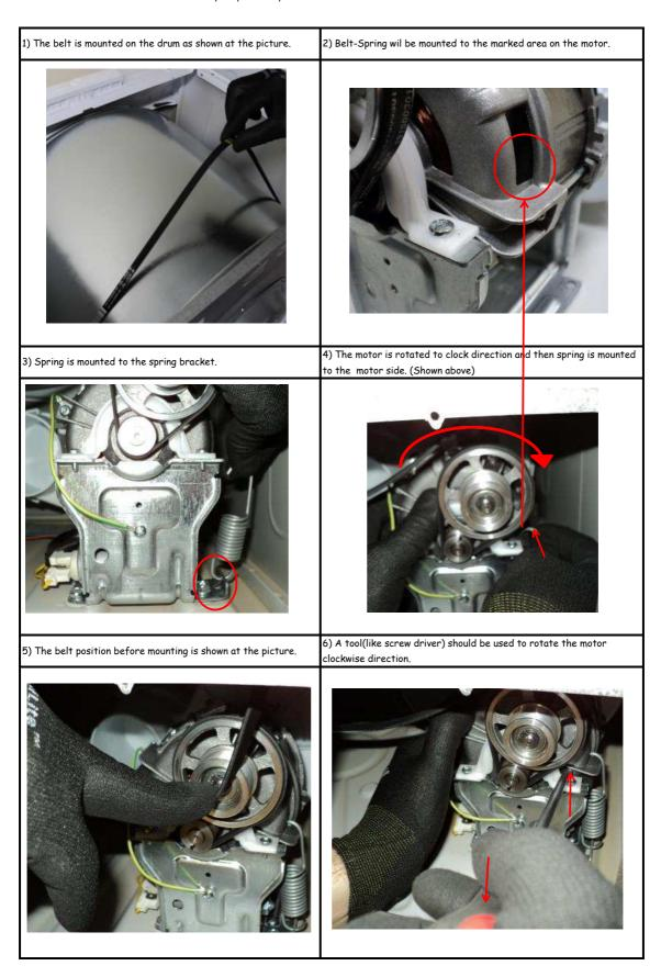
7) The next mounting step using a tool is shown at the picture. The belt should be fitted on the pulley.
