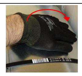
11) After rotating the drum the belt position on the pulley is shown at the picture. Two grooves shuld be left at right side as shown at the picture.
