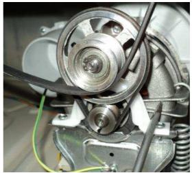
9) The belt should be mounted to the pulley as in the picture.
