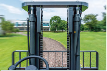
Wide field of vision mast improves the safety of stacking operations.
