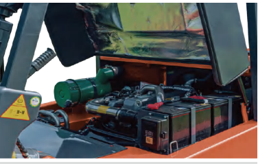
The hood opening angle is increased to 80°, making maintenance more convenient.
