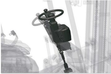
The steering wheel angle is adjustable, Applicable to a wide range of people.
