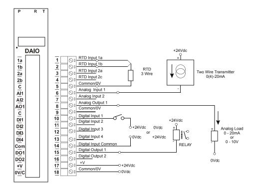
The following diagram shows how the inputs and outputs are connected to the DAIO module.
