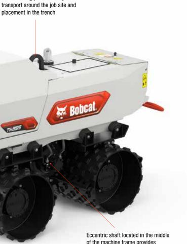
of the machine frame provides unprecedented compaction output
