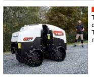
DUAL AMPLITUDE Two amplitude settings and centrifugal weights allow the TR75 to excel on a range of materials and job sites.
