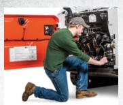
The service schedule inside the rear door provides service and maintenance instructions. Lubricate, grease and check fluid levels on the loader as required. Check for leaks and broken or damaged parts before operating.
