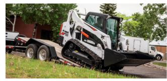
Always drive up the ramp with the heavy end uphill. With an empty bucket or no attachment. the rear of the machine is heavier. Engage the parking brake.
