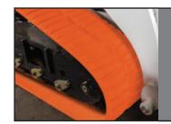
Optional non-marking multi-bar lug rubber tracks won't leave black rubber marks on hard surfaces like concrete.
