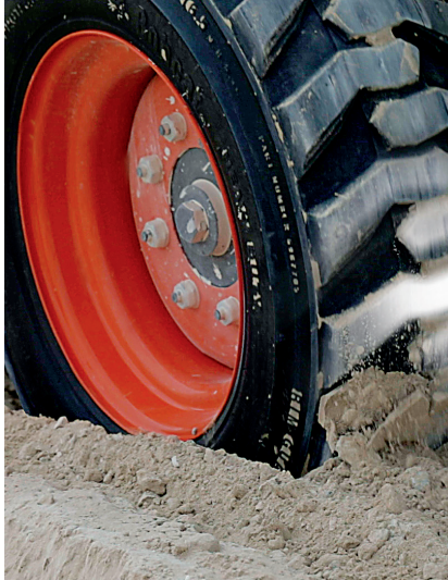
CURVED LUGS IMPROVING TIRE CLEAN-OUT
