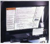
The service schedule under the hood provides service and maintenance instructions. Check fluid levels, lubricate and grease the machine as required. Check for leaks and broken or damaged parts before operating.
