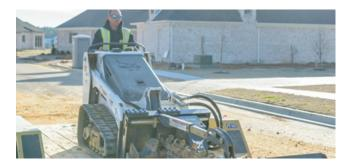
Always drive up the ramp with the heavy end uphill. With an empty bucket or no attachment, the rear of the machine is heavier. Engage the parking brake. Secure the loader and attachments to the tie-down points using chains and binders (see Operation & Maintenance Manual for more details). Use a towing vehicle and trailer of adequate capacity.
