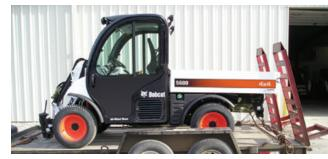
Always drive up the ramp with the heavy end uphill. Place the travel direction control
