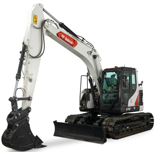
With its turbocharged 3.4 liter, non-DPF engine and class-leading hydraulics, the new Bobcat® E145 delivers a mighty combination of maneuverable size, high lifting capability and powerful breakout forces for prolific digging performance.
