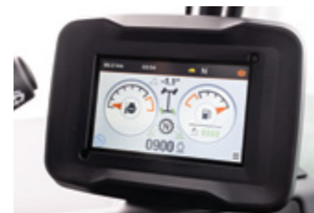
5" LCD display with navigation jog shuttle
