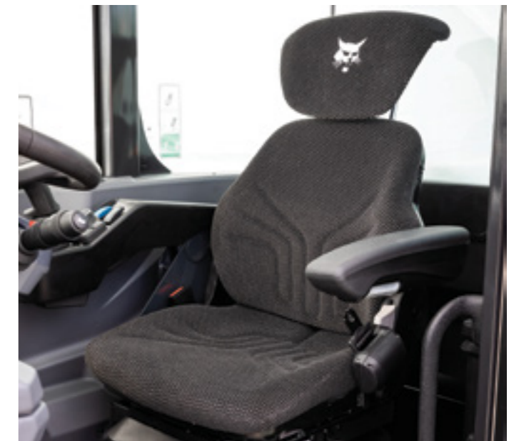
Grammer Maximo Air suspended seat with heating, Dynamic Dumping System (DDS) and joystick mounted on suspended armrest
