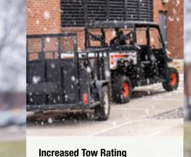
The tow rating has increased by 25%, and the trailer hitch tongue weight rating is now 250 pounds (113 kg), giving you a powerful option for pulling heavy trailers and other equipment for the job. Haul up to 2,500 pounds (1134 kg) with confidence.
