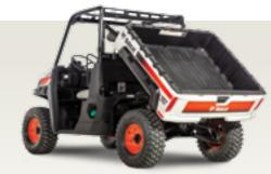
large, heavy objects. A convenient, single-latch tailgate secures your load, allows for odd-shaped cargo and allows for easy loading and dumping.
