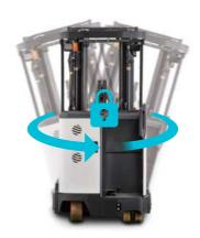
It automatically locks the suspension while starting, turning, and mast operating to increase stability. Thus it makes job more safe and comfortable during driving or cargo handling.
