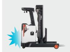
► FRONT PROTECTOR (OPTION) By applying front protector, operator is protected from external threats such as falling objects.
