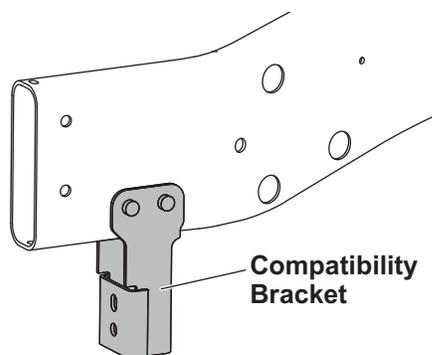
3. Remove the nuts from the bumper fastener assembly on both sides of the vehicle. For both driver-side and passenger-side mounts, align the forward mount holes with the protruding cap screws and guide the mounts onto the respective fastener assembly. Loosely fasten by reinstalling the original nuts.
