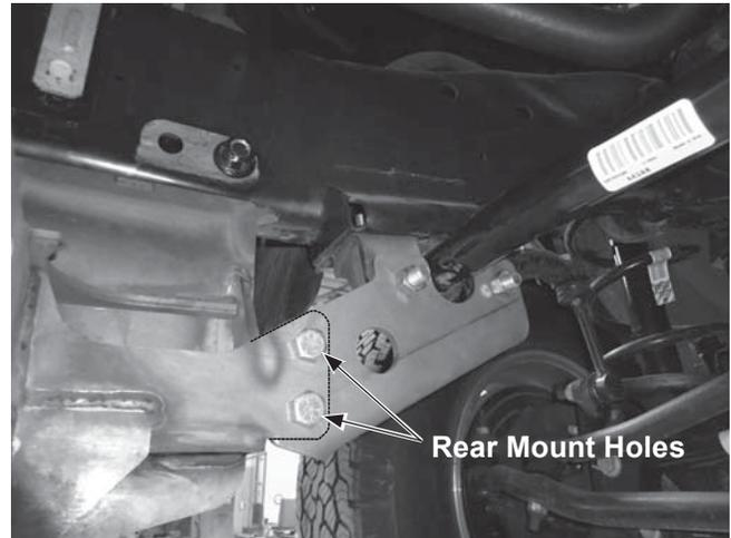
**Thrust arms are interchangeable and can install on either side of the vehicle. There is no left or right side-specific part.**
