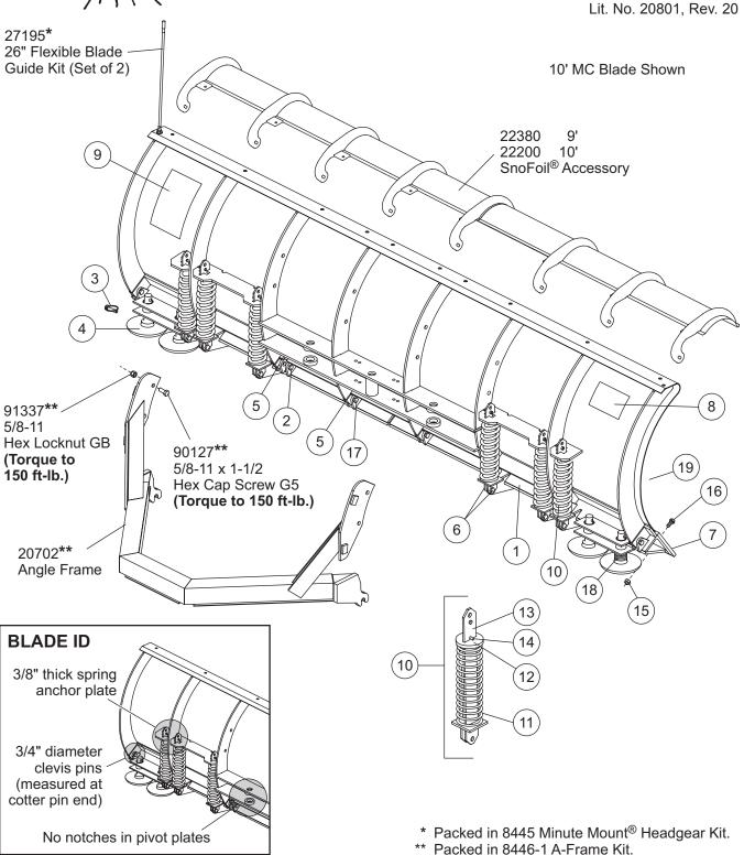
This parts list is for FISHER® MC Series Blades produced before September 2001.
