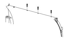
Place the rubber deflector with the logo on it on top of the moldboard and align the first hole in the deflector with the outermost hole in the moldboard. The deflector will extend beyond the end of the wing on 7-1/2' and 8-1/2' models.
