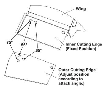
**HD2™ Snowplow:** Align the holes in the cutting edges with the holes in the wing base angle that correspond to the 55° attack angle setting.
