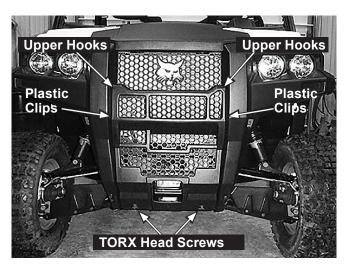
3. Position the skid plate assembly as shown.
