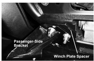
If the vehicle is equipped with a winch: Align one hole in the winch plate spacer with the bottom hole of the passenger-side bracket to fill the existing gap. Install the bracket and spacer using two 3/8" x 1-1/2" carriage bolts and 3/8" locknuts. (The second hole in the spacer is not used.)
