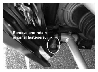
2. Install the mount skid plate assembly as shown. Reuse the OEM fasteners removed in Step 1 in the front holes. Use the supplied 3/8" x 1-1/4" cap screws in the remaining four positions. Fasteners should be finger tight.
