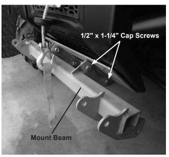
Measure the distance between the mount beam rear hole and the ground. If it exceeds 11-1/2", install the accessory Adapter Plates Kit (PN 77555) to ensure optimum plowing performance.
