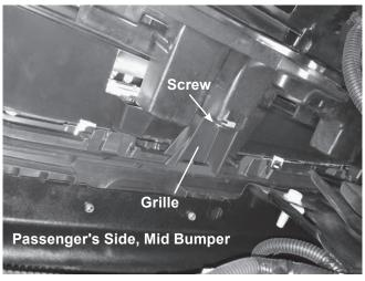
Remove the two bumper cover screws located on the inside of each front wheel well. If the vehicle is equipped with fender trim, it will need to be displaced in order to access the screws.
