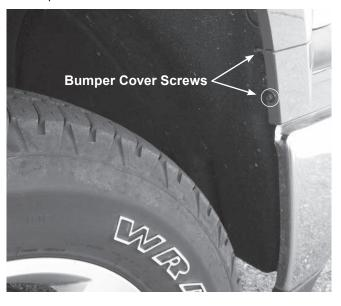
5. Release the hidden locking tabs on each side of the vehicle and pull the bumper cover outward.
