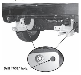
Using the rear holes in the passenger-side mount as a guide, drill two 17/32" holes into the truck frame.
