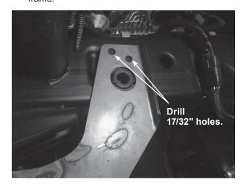
Insert two 1/2" x 1-1/2" cap screws with handles and 1/2" flat washers into the inside of the truck frame and out through the rear drilled holes. Attach a 1/2" locknut to each cap screw and hand tighten.
