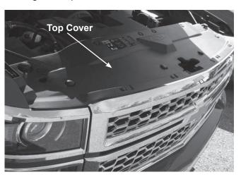
2. Remove the four cap screws and release the locking tabs located along the top of the grille.
