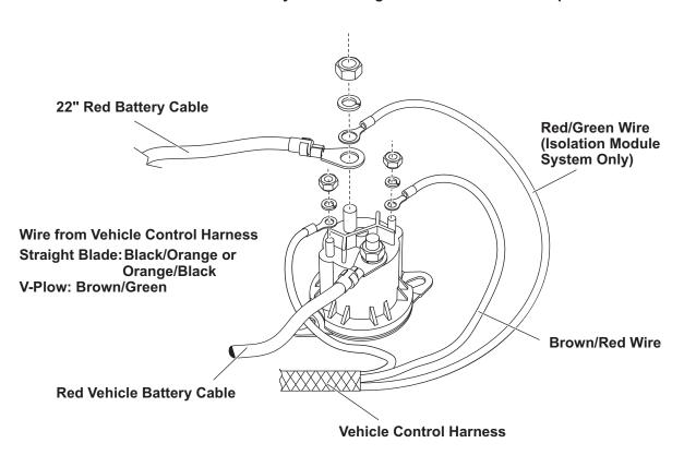
Non-FLEET FLEX Electrical System – Straight Blade and MVP<sup>®</sup> Snowplows
