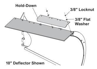
5. Install one 3/8" flat washer and 3/8" locknut on top of the outermost cap screw and hand tighten. Repeat for the second cap screw.
