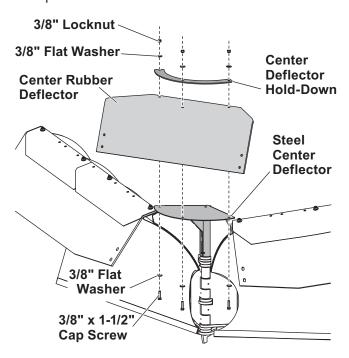
2. Attach the center rubber deflector to the wing rubber deflectors using the provided 3/8" x 1-1/2" cap screws, 3/8" flat washers, and 3/8" locknuts in the pre-made holes.
