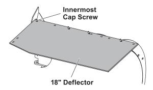
4. Place one hold-down over the deflector, with the outermost cap screw through the outermost hold-down hole.
