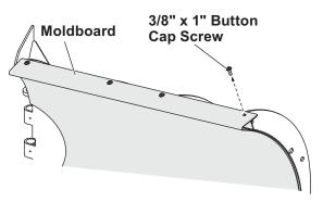
Install the supplied 3/8" x 1-1/2" cap screws and 3/8" flat washers through the blade frame and the moldboard from the bottom up. Install a second 3/8" flat washer and 3/8" locknut to each cap screw and tighten.
