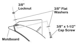
NOTE: On 7'6" and 8'6" blades, the deflector will overhang one end of the wing as shown.
