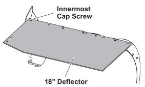
4. Place one hold-down over the deflector, with the outermost cap screw through the outermost hold-down hole.
