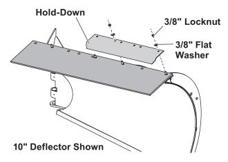
Install one 3/8" flat washer and 3/8" locknut on top of the outermost cap screw and hand tighten. Repeat for the second cap screw.  Place a second hold-down over the deflector, with the innermost cap screw through the innermost hold-down hole. The hold-downs may overlap. Install one 3/8" flat washer and 3/8" locknut on each cap screw attaching the second hold-down.
