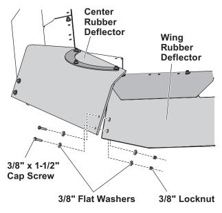
NOTE: It is normal for the rubber center deflector to bunch up when the blade is angled or moved into the scoop position.
