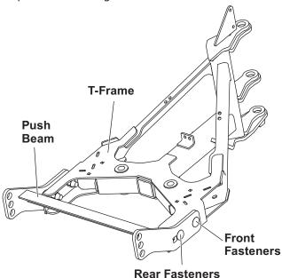
Select the hole in the rear of the T-frame that is aligned closest to the rear holes in the pushbeam. Reassemble the previously removed fasteners into the rear holes.
