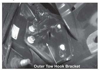
Remove the compatibility brackets from the frame, if so equipped (see illustration below). Save the brackets and hardware for the vehicle owner.
