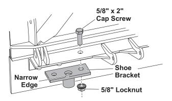
2. Align the edge of the shoe bracket with the edge of the base angle and clamp in place. Using the holes in the bracket as a guide, drill one 1-1/16" hole and one 11/16" hole in the base angle, as shown below.
