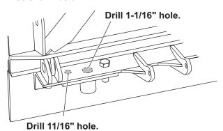
3. Insert a 5/8" x 2" cap screw down through the outermost hole in the base angle and the shoe bracket. Attach a 5/8" locknut and tighten both fasteners to 150 ft-lb.
