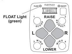
Pressing the four diamond-shaped buttons in the center of the control face will result in the blade movements described in the following table.
