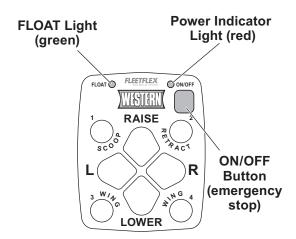
Buttons numbered 1, 2, 3, and 4 control SECURITY GUARD™ system functions.
