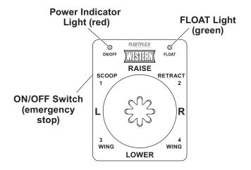
Positions numbered 1, 2, 3, and 4 control SECURITY GUARD™ system functions.
