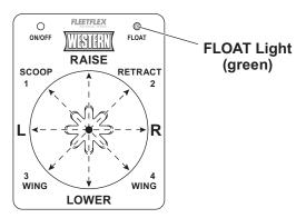
Moving the control lever straight up and down or from side to side on the control body will result in the blade movements described in the following table.
