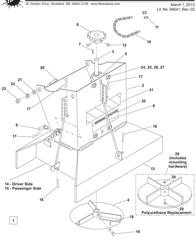
This parts list is for FISHER® Hopper Spreaders with serial numbers 4809 and higher.
