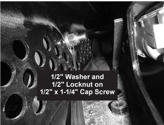
14. With the help of another person, reinstall the bumper. Trim the plastic air dam as necessary to install the mount beam between the passengerand driver-side hanger assemblies. Insert 1/2" x 1-1/4" cap screws through the hanger assemblies and the mount beam (8 total). Secure each fastener with a 1/2" locknut. Hand tighten.
