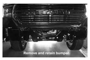
3. Beginning on the passenger's side, remove and set aside the tow-hook bolt and small washer. Remove the large tow-hook washers, isolator, and tow hook and retain these parts for reinstallation if the mount is removed. Reinstall the small tow-hook washer and bolt. Torque fastener according to the torque chart.
