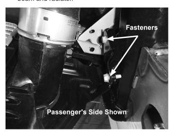
16. Install the thrust arms to the rear thrust assembly using 1/2" x 1-1/4" cap screws. Secure the thrust arms to the rear tabs of the mount beam in a similar fashion.
