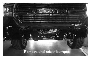
3. Beginning on the passenger's side, remove and set aside the tow-hook bolt and small washer. Remove the large tow-hook washers, isolator, and tow hook and retain these parts for reinstallation if the mount is removed. Reinstall the small tow-hook washer and bolt. Torque fastener according to the torque chart.
