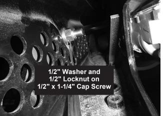
14. With the help of another person, reinstall the bumper. Trim the plastic air dam as necessary to install the mount beam between the passenger- and driver-side hanger assemblies.2025 and newer model years might require more trimming to the metal portion of the bumper.
