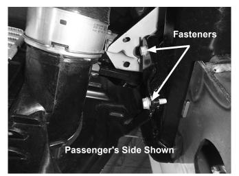
16. Install the thrust arms to the rear thrust assembly using 1/2" x 1-1/4" cap screws. Secure the thrust arms to the rear tabs of the mount beam in a similar fashion.
