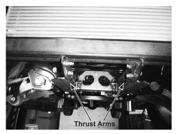
17. Tighten all fasteners according to the torque chart.
