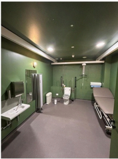
Changing Places Toilet (Adult changing surface, hoist, privacy screen, support rails, emergency cord)
