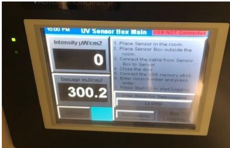
Figure 14 – Run cycle until dose is not less than 300 mJ/cm 2 .
