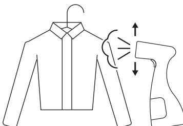
**NOTE:** the clothes steamer is designed to be used in an upright position on hanging garments. For occasional touch ups the steamer can be used in a horizontal position.
