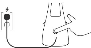
Once filled with water, connect the electrical cord ⑨ to your power supply then press the power button ⑦ on the back of the steamer.
