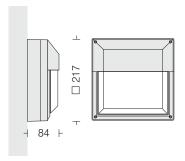
Icecube 5L LDW0583 12 Power 12W LED Housing & Cover Plate Diffuser 3000K
