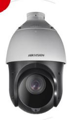
Hikvision DS-2DE4215IW-DE (E) 2MP 15× Network IR Speed Dome adopts 1/2.8" progressive scan CMOS chip. With the 15× optical zoom lens, the camera offers more details over expansive areas.
