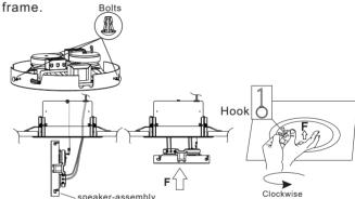
5. Disassembly process: one hand to hold the speaker assembly and push it up slightly, then use a hook to hook the edge of grill and rotate counterclockwise till the speaker assembly apart from the frame.
