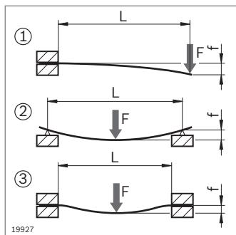
$$f_{(1)} = \frac{F \times L^3}{3 E \times I \times 10^4} \quad \text{Profile deflection due to force } F \text{ for static load cases } ①②③$$
