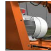
22 kW Electric motor Power for softwoods and hardwoods.
