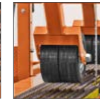
Two Roller Hold-downs Wide hold-down rollers keep the cant stable during cutting.
