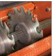
2 Circular Blades One fixed and the other fully adjustable.
