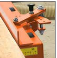
Adjustable Fence Allows you to quickly position boards that already have one straight edge.
