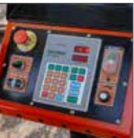
Standard Networks Rugged electronics quickly position the adjustable blade to precise measurements.
