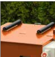
Top rollers Make it easy to return boards that require a second pass.
