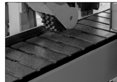
Infeed Hold Down Roller Heavy duty driven roller on infeed.
