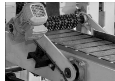
Outfeed Hold Down Roller Heavy duty driven roller on outfeed.
