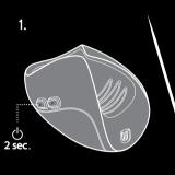
Before use, hold (power button) for 2 seconds. PULSE enters into Bluetooth mode for 30 seconds.
