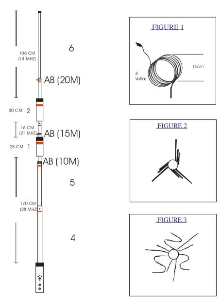
2.1 - Place element 5 inside element 4 (base), 2 in 1 (traps), 1 in 5 and 6 in 2.
