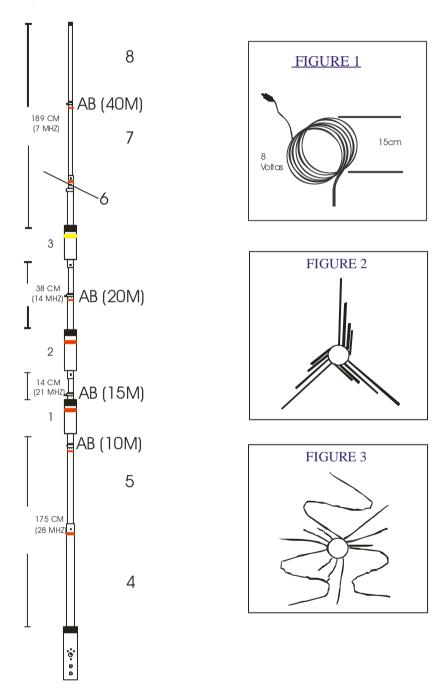
$2.1 - Place \ element \ 5 \ inside \ element \ 4 \ (base), \ 3 \ in \ 2, \ 2 \ in \ 1 \ (traps), \ 1 \ in \ 5, \ 6 \ in \ 7, \ 7 \ in \ 3 \ and \ 8 \ in \ 7.$
