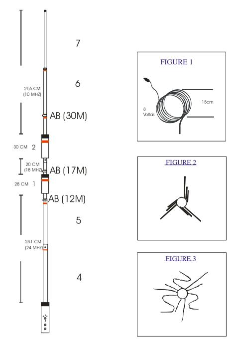
2.1 - Place element 5 inside element 4 (base), 2 in 1 (traps), 1 in 5, 6 in 2 and 7 in the 6 Follow the starting lengths in the drawing.
