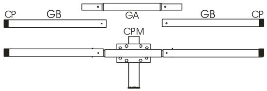
Fixing the element to the boom:
