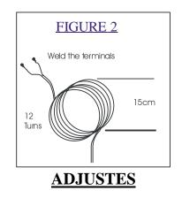
If there is a need for adjustments, make small adjustments to the element in 1 band at a time starting at 10m and then at 15, 20 and finally 40m, increasing if you want to lower the resonance frequency or decreasing if you want to up the resonance frequency, as the adjustment of one band can interfere with the adjustment of another band, always mark what you are doing and then put the same measurement on the other side of the antenna.
