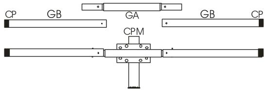
Fixing the element to the boom:
