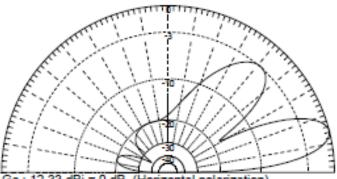
Ga: 12.33 dBi = 0 dB (Horizontal polarization) F/B: 19.95 dB; Rear: Azim. 120 deg, Elev. 60 deg
