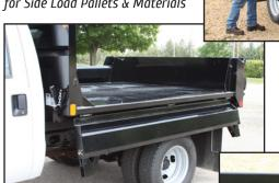
Fold Down Sides with Quick Latch System
