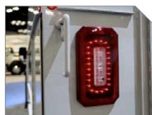
**N** Upgraded surface mount lighting system features LED S/T/T and B/U, LED strobe option with (9) selectable patterns, and built-in reflectivity for additional safety
