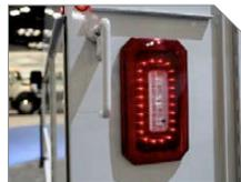
**I** Upgraded surface mount lighting system features LED S/T/T and B/U, LED strobe option with (9) selectable patterns, and built-in reflectivity for additional safety
