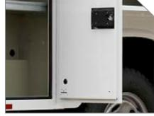
**H** Features double-shell, 20-gauge, two-sided A-40 galvalneal steel compartment doors
