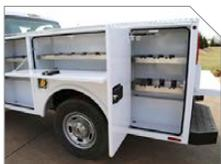
**E** Inset door frame design with double tray aluminum doors and neoprene seals for weather-tight closing
