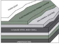
**A** Features 14-gauge, two-sided A-40 galvalneal steel shell
